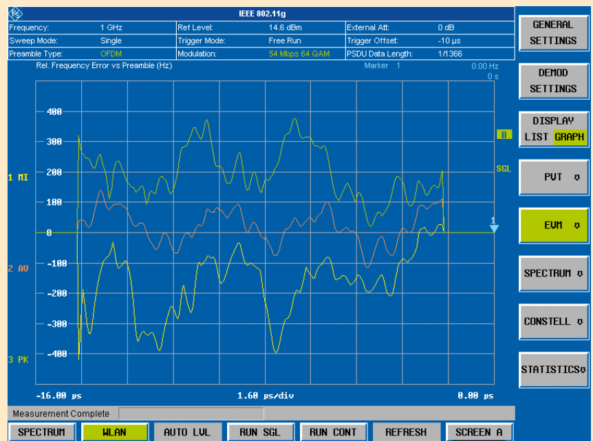
FIG 2 A special frequency/phase error measurement displays the frequency and phase characteristic at the beginning of the burst (in the preamble).
