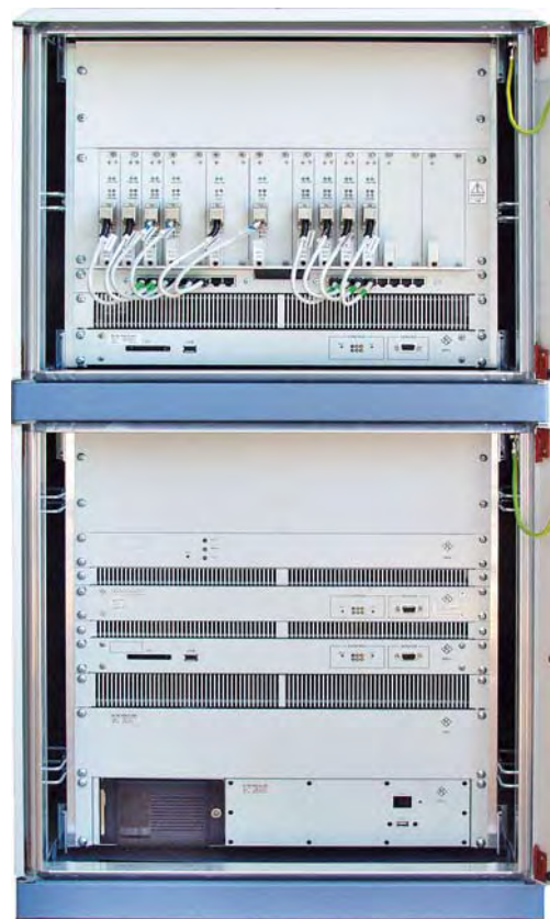
FIG 4 The R&S ® IpSN system node is a cascadable 19" standard block.
