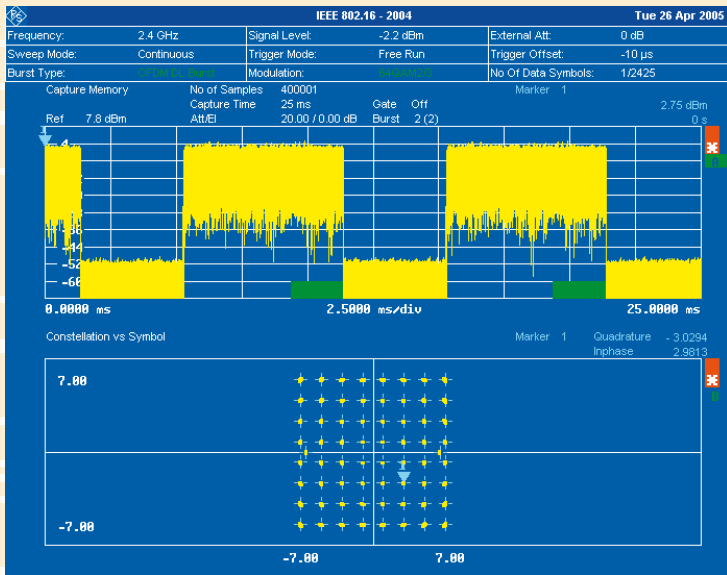
FIG 5 WiMAX signal with constellation diagram. The 64QAM burst parts highlighted in green are demodulated and results shown in the constellation diagram.
