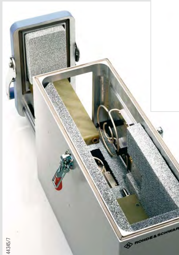
FIG 4 Interior view of R&S®TS7121A with GSM antenna coupler and supporting plate.
